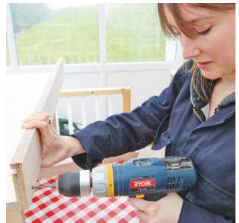
▲ Pic.12 Piloting by hand: Imogen is watching the bubble on the drill so as to hold it horizontally. "Here we screwed not into the middle of the ply but into the middle of the tongue, so accuracy was important. Working on a breakfast table is far from ideal"
